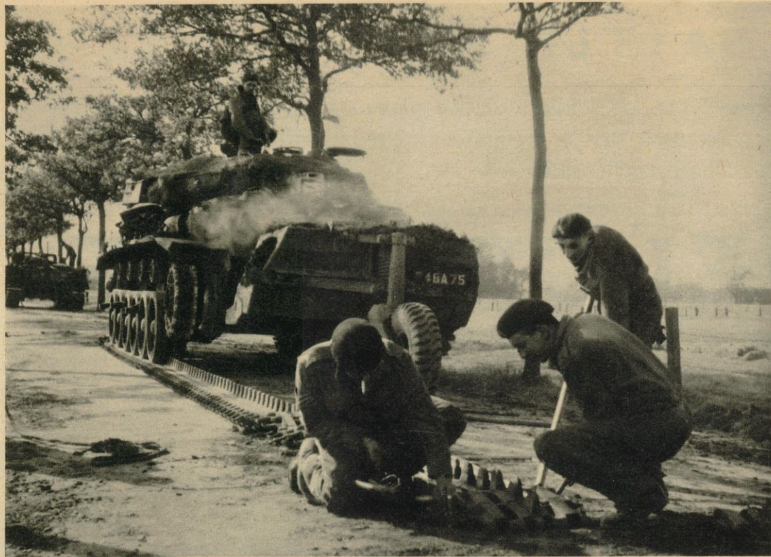
A tank crew of 6th Royal Tank Regiment repair a broken track.
