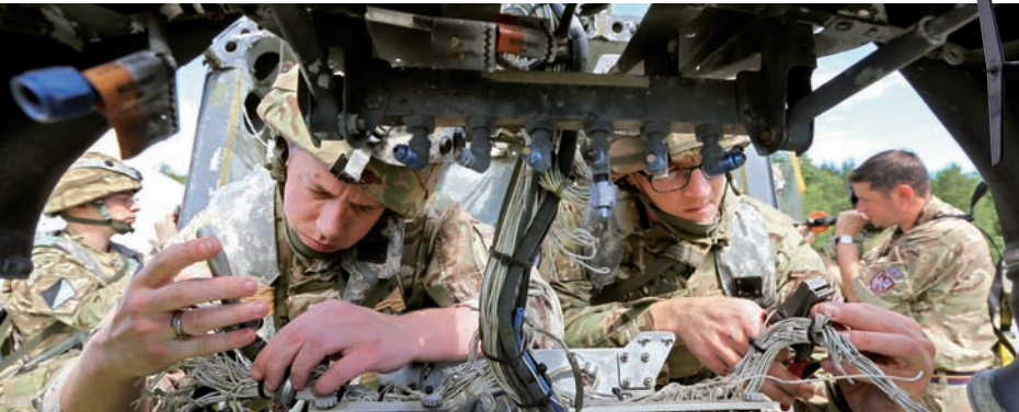
Make do and mend: Sgt Luke Morris and LCpl Christopher Cartwright (both REME) carry out battlefield repairs on a disused helicopter
