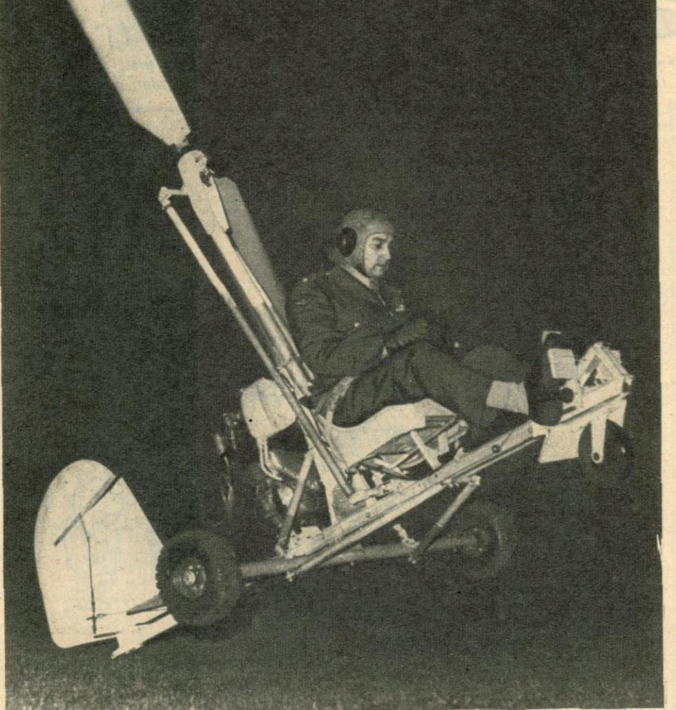
As the rotor blades turn the Reccecopter, with Major N. A. Edwards at the controls, rises from Gordon Barracks. The frame is of aluminium and the machine is powered by a motor-cycle engine.
