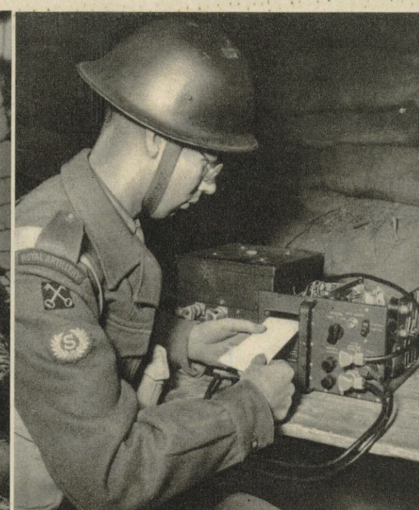
On the sensitized paper in this recorder four electrical pens, linked to the microphones, scratch tell-tale marks.
