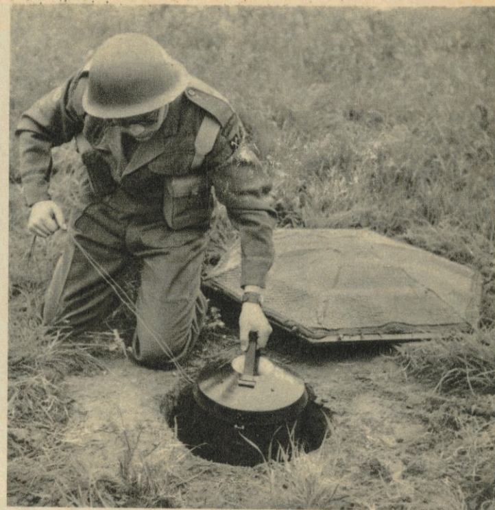
The microphone—looking like a small metal hat-box—is lowered into the ground. It is covered with a hessian net to eliminate wind interference.
