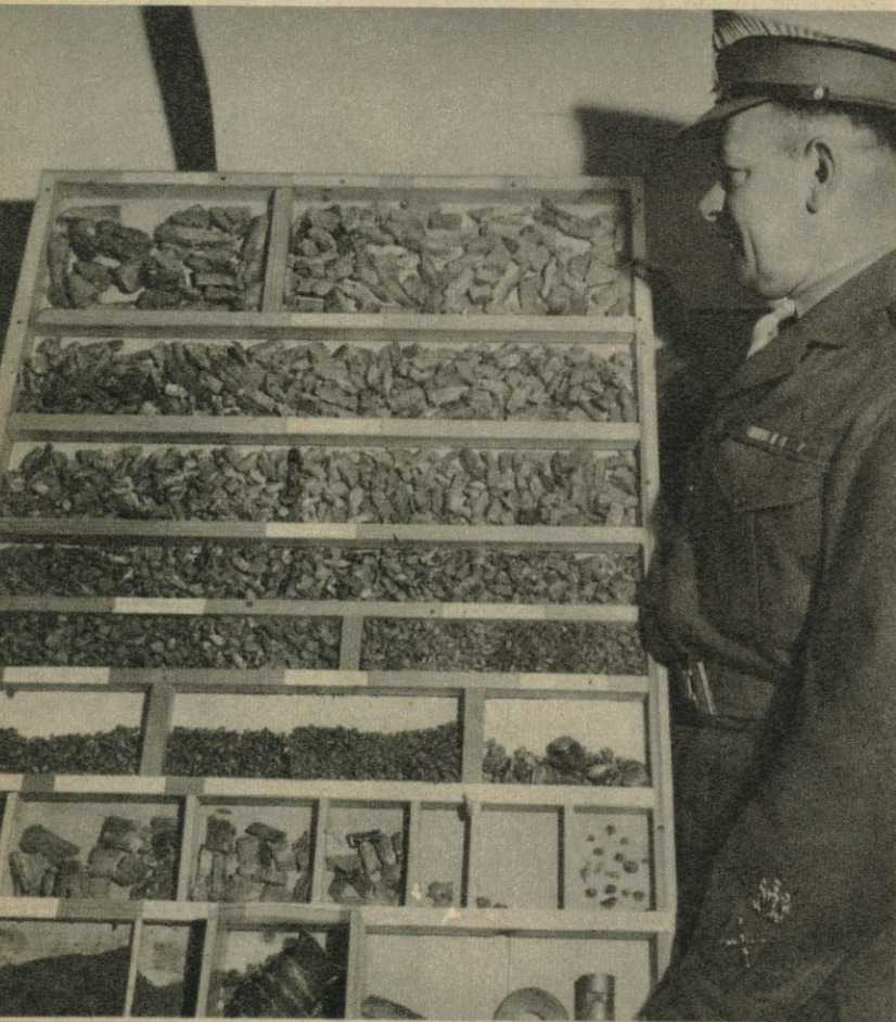
Serjeant-Major Instructor in Gunnery J. A. Hambidge (Manorbier's senior warrant-officer instructor) displays a case showing the fragmentation of a 5.25 round. This one was exploded in sand, and the pieces carefully collected. They range from big lumps (top) to near-powder (bottom). A round which wholly disintegrated into powder would not be destructive enough; nor would one which exploded into only half a dozen big lumps.
