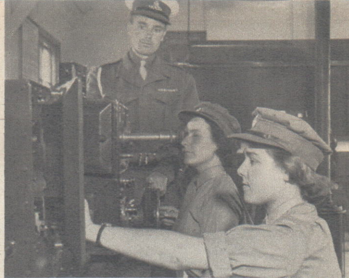
Left: L/Cpl. W. P. Smith WRAC trains Privates J. P. Webb (left) and C. Doherty, on the kine-theodolite, for observing bursts.
