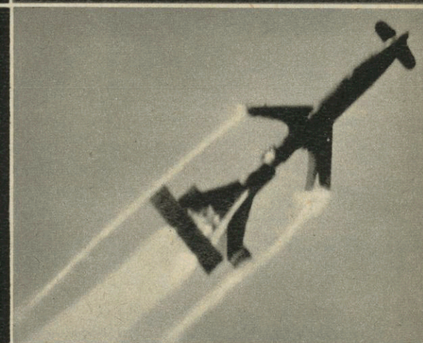
Like the British rocket pictured on Page five, the Rheintochter was a boosted missile. The boost section fell away when the main propellant was fully ignited.
