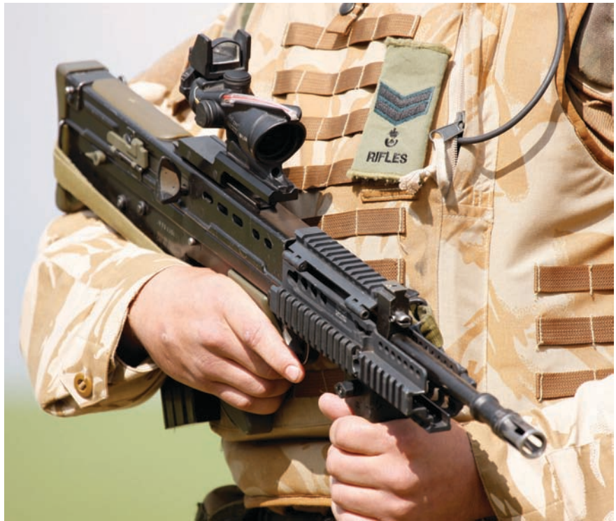
Cornering problems?: The British Army's SA80 A2, pictured above with improved stock and hand grip (which also contains a drop out bipod), and featuring the advanced optical gunsight Picture: Steve Dock
