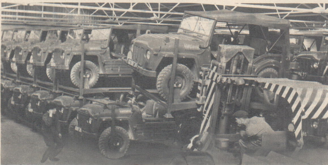
Below: A fork-lift truck doubles stacks of Champs to save storage space. Each vehicle is secured in a steel pallet.
