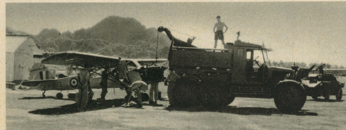
With the help of a 12th Royal Lancers' "wrecker," an Auster engine is changed on an outlying airstrip.
