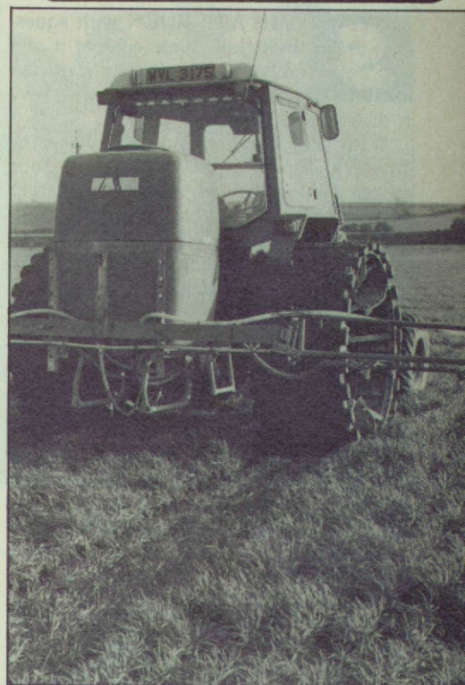
Demonstration in a Lincolnshire field shows how wide wheels make only a shallow depression. ▲
