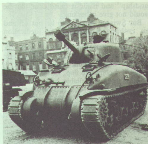
Best-known last war tank—the American Sherman. Carried 75mm gun, 3-inch armour, 25mph.
