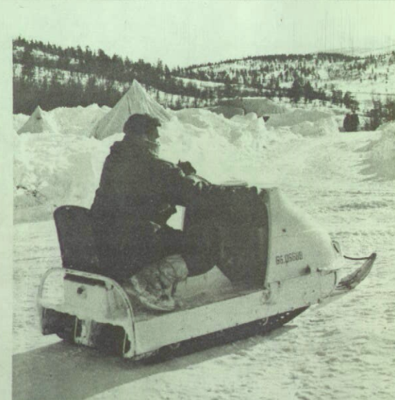
Above: A Canadian returns to camp on a Ski-do, a tracked cross-country snow scooter powered by a two-stroke engine.
