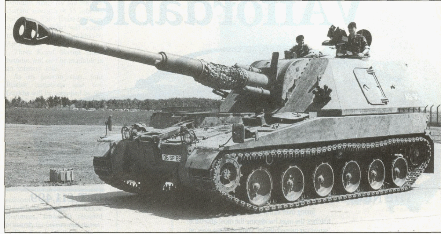
AS90, the powerful 155mm self-propelled howitzer which enters service next year
