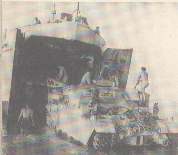
This powerful armoured recovery vehicle helps to unload equipment from a tank landing craft. Below: The light but powerful 105mm howitzers are quickly in action to repel an enemy thrust.
