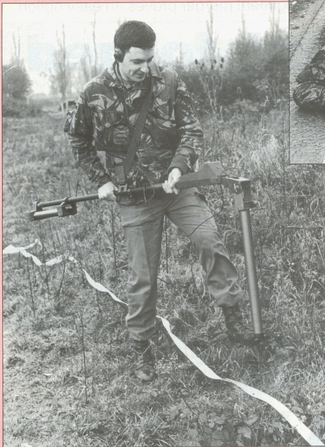
A TA sapper uses a sensitive electronic locator to pinpoint unexploded mines
