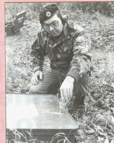
Sgt Paul Mayle uses a microphone stethoscope to listen to a suspect device. The sensitive mike can pick up sounds like the ticking of clockwork, mechanisms and even the hiss of escaping rocket fuels
