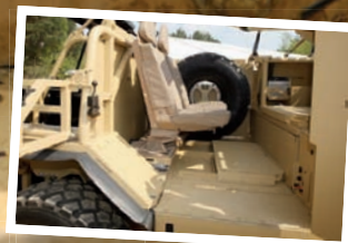
Doors hinged to open up to 180 degrees to improve access and allow space for a stretcher
