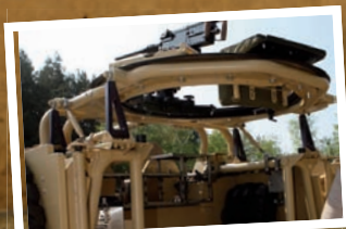
Gunner's ring mount moved to reduce muzzle blast
