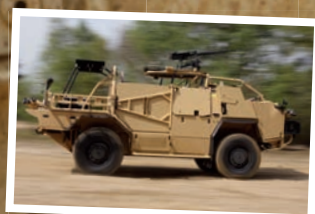
Jackal 2 has a 6.7 litre engine, is 14 inches longer and has a vehicle-powered Bowman communication system
