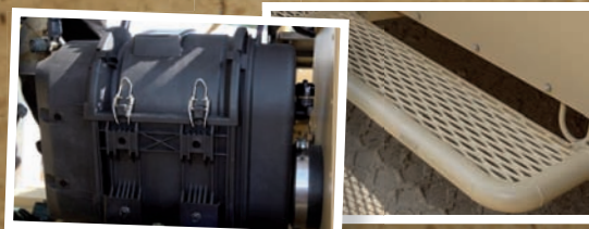
Improved air filter system and a step installed to ease dismounting
