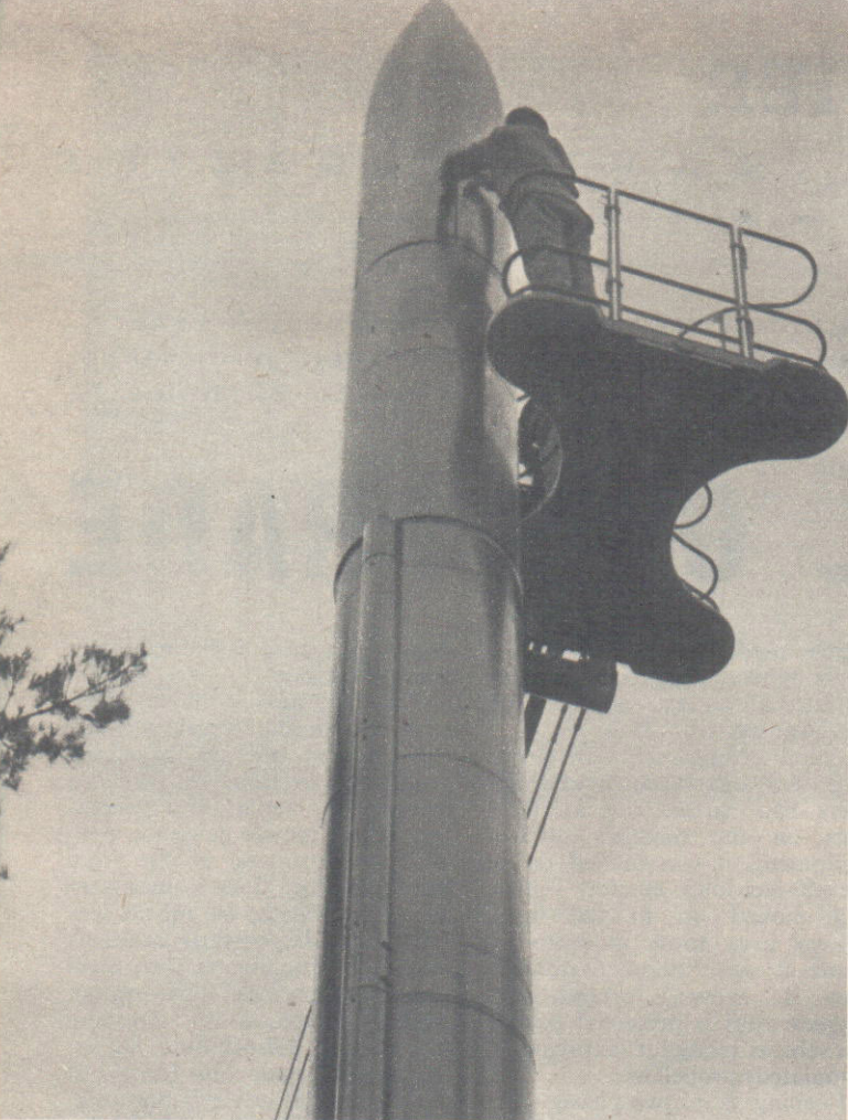
Above: The "cherry picker" hoists a technician aloft for last-minute adjustments to the rocket mechanism. Below: The Corporal on its launcher. Note the soil placed over the legs of the launcher—to protect paintwork from the heat of take-off!
