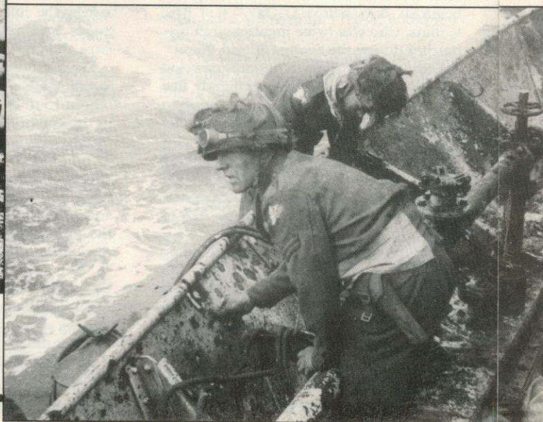
Below – After just one Crab flail tank got ashore from LCT 947, two direct hits knocked out a second and detonated Bangalore torpedoes, killing the commanding officer of 5 Assault Regiment RE, Lt Col A D B Cocks, and others. Unable to discharge its cargo, the craft withdrew and sailed back to England, carrying its dead and wounded with it. Here, sappers are seen plugging shrapnel holes
