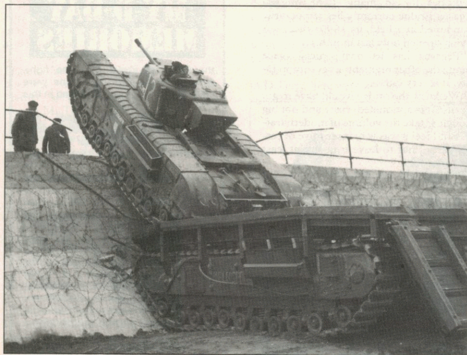
This photograph of an "Ark" bridge tank was not released until exactly one year after the original D-Day landings. In this trial, the Ark formed a ramp up which armoured vehicles were able to advance to scale obstacles such as sea walls
