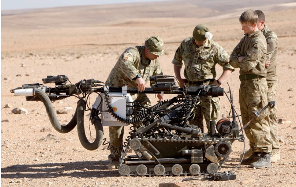
Pashtun preparations: LCpl Paul Armbuster (RLC), a destroyer-operator with 11 EOD Regiment, shows colleagues from other British Army units how the remote-controlled Wheelbarrow 8B EOD robot functions
