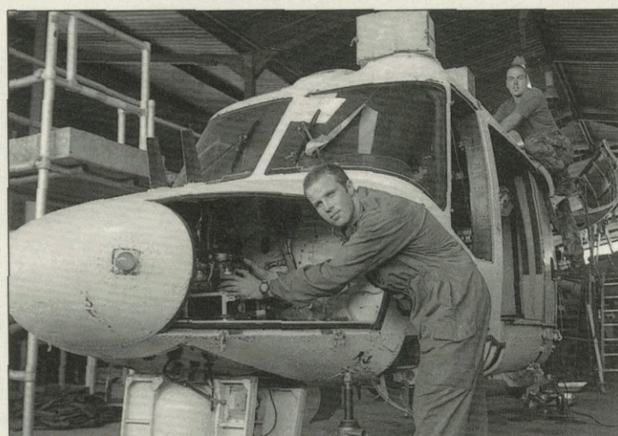
LCpl Will Watchorn (front) and Stuart Leadbeater carry out the first 800-hour service under operational conditions on an AAC helicopter
