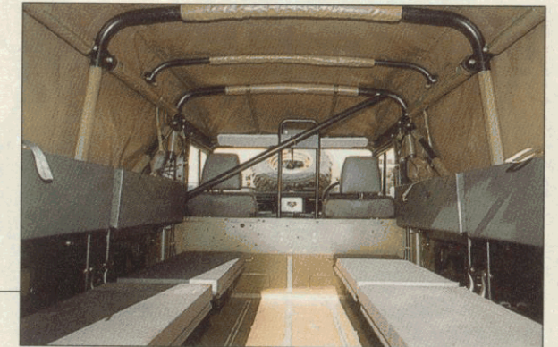
Above – A new roll bar system and better seating in the rear of the vehicle offers increased passenger safety and comfort. The MoD has taken up an option of rear seat belts on every vehicle
