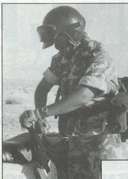
Rapid response dispatch rider Cpl Stan Hogg of 1 PC Regt RE has fixed a metal holster to his 500 cc Armstrong to hold the Sterling sub-machine gun he carries. It is possible to extract the weapon and load it while driving with one hand
