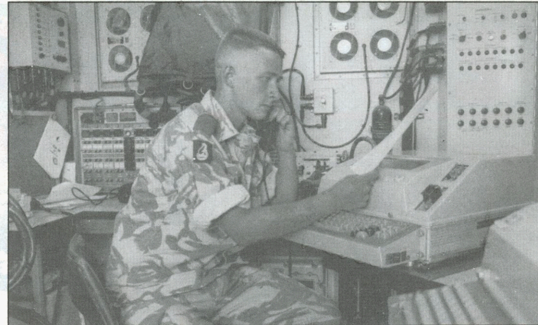
Cpl Clive Kitchener mans a Ptarmigan secondary access switch and message centre
