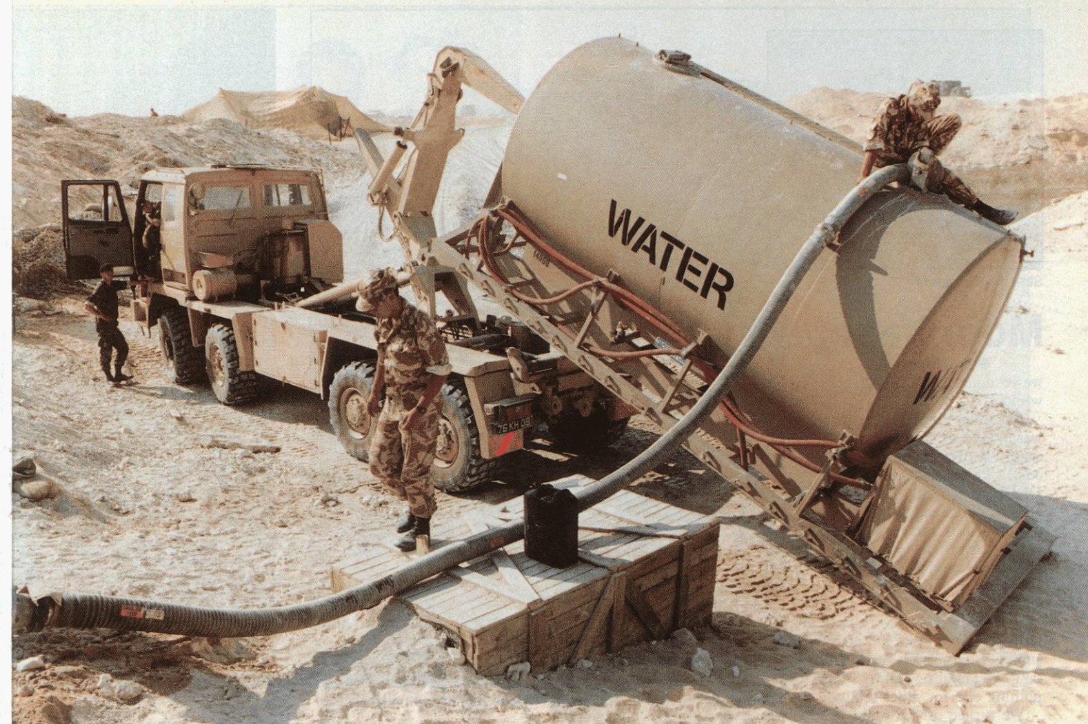
DROPS makes the delivery of water by "bean can" to a supply point in the desert that much easier
