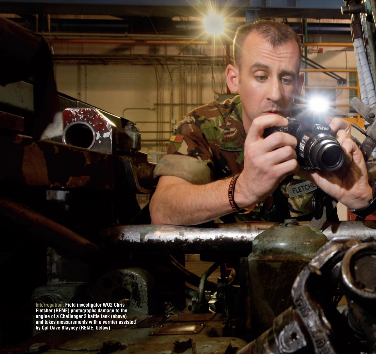
**Interrogation:** Field investigator WO2 Chris Fletcher (REME) photographs damage to the engine of a Challenger 2 battle tank (above) and takes measurements with a vernier assisted by Cpl Dave Blayney (REME, below)
