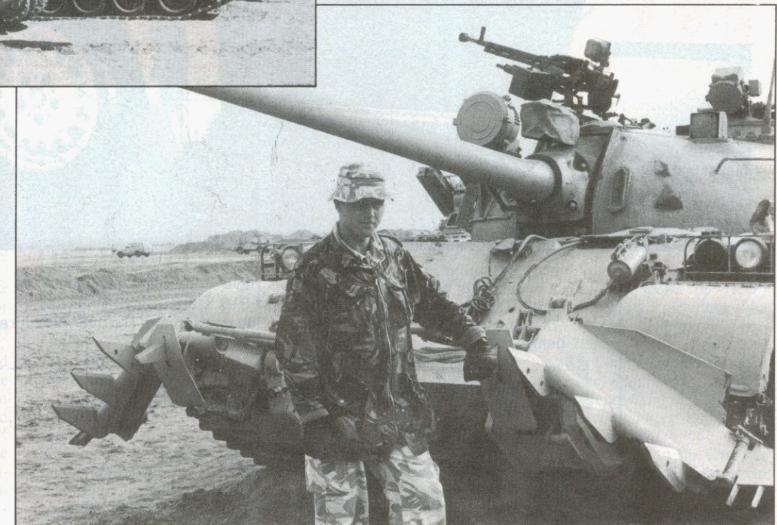
Cpl Chris Barton of 1st Fd Sqn, 21 Engr Regt, inspects a Chinese-manufactured Type-59 tank. It is fitted with a KMT6 mine plough
