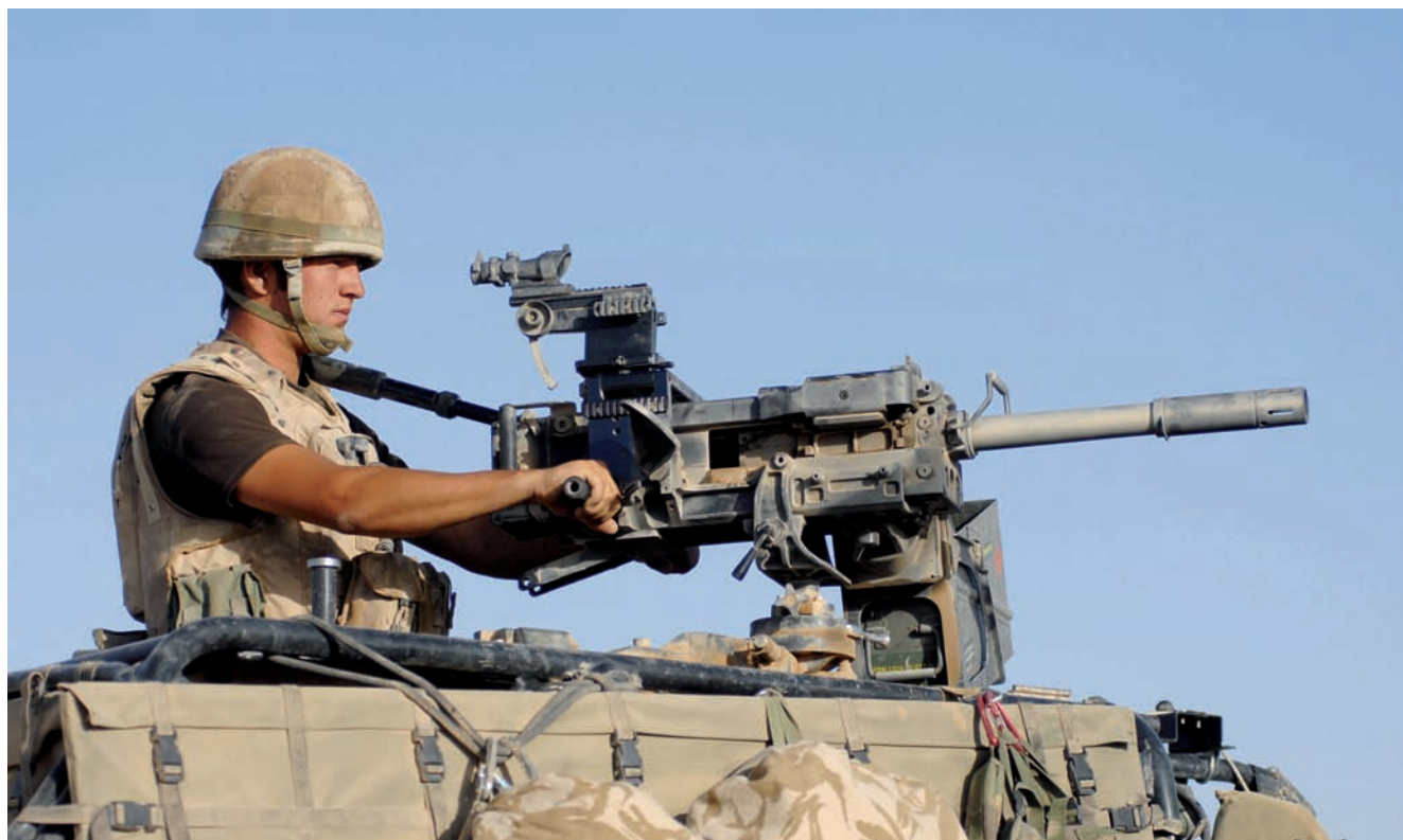
Packing a punch: Capable of firing 340 high explosive rounds a minute, the grenade machine gun has already seen action against the Taliban in Afghanistan
