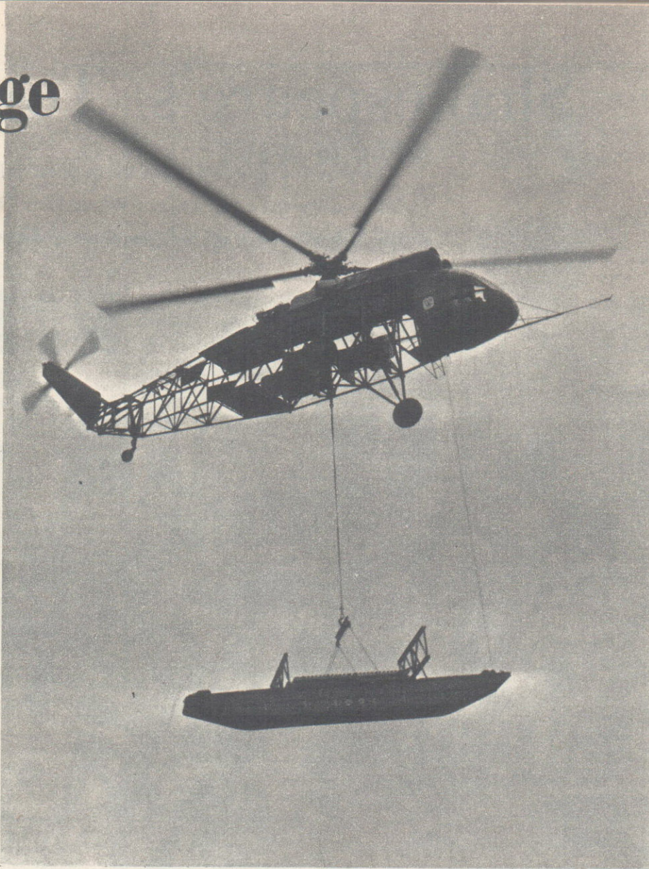
Above: A three-ton pontoon is well within the lifting capacity of the Westminster which cruises at 80 knots with a slung load.
