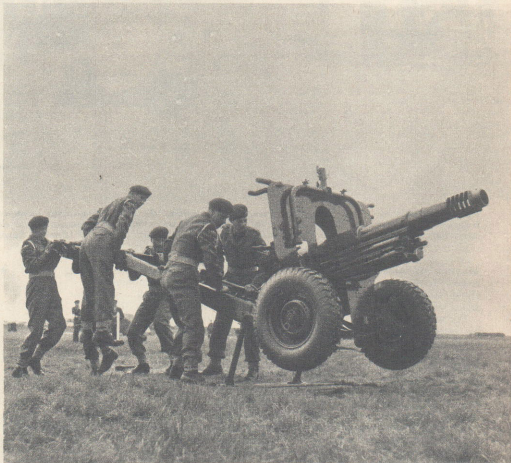
Below: The 105-mm. pack howitzer is easily manageable by its six-man detachment here seen straightening its adjustable legs for the anti-tank firing position. The howitzer can also be used as a mortar.
