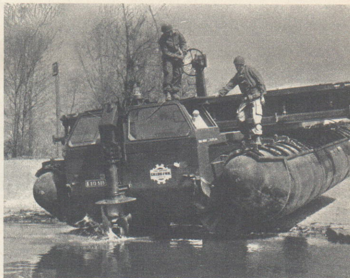
With its decking in position, one of the floating bridge vehicles enters the water. When afloat the wheels retract and the propeller takes over. Below: Laden with a 65-ton Conqueror, the Gillois bridge swims down river.
