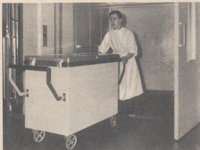
Food wagons are plugged into the electric mains in the kitchens — and again in the wards. As a result food is always hot.
