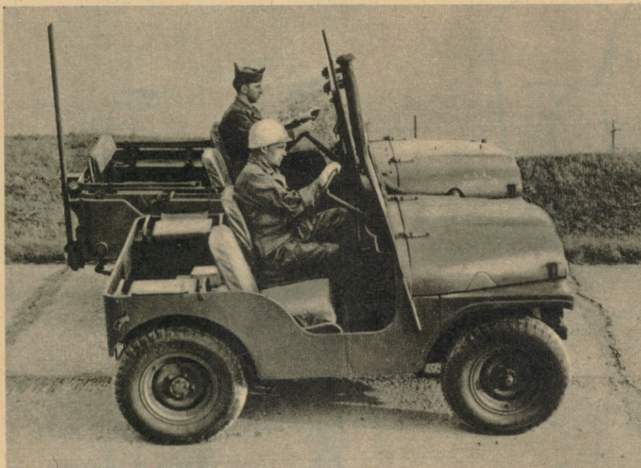
Developed for airborne use: the new shorter jeep seen against the standard model.
