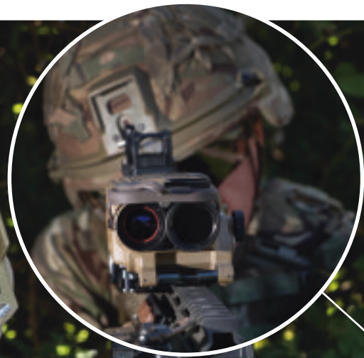
A full picatinny rail allowing the fitment of the in-line low light sight
