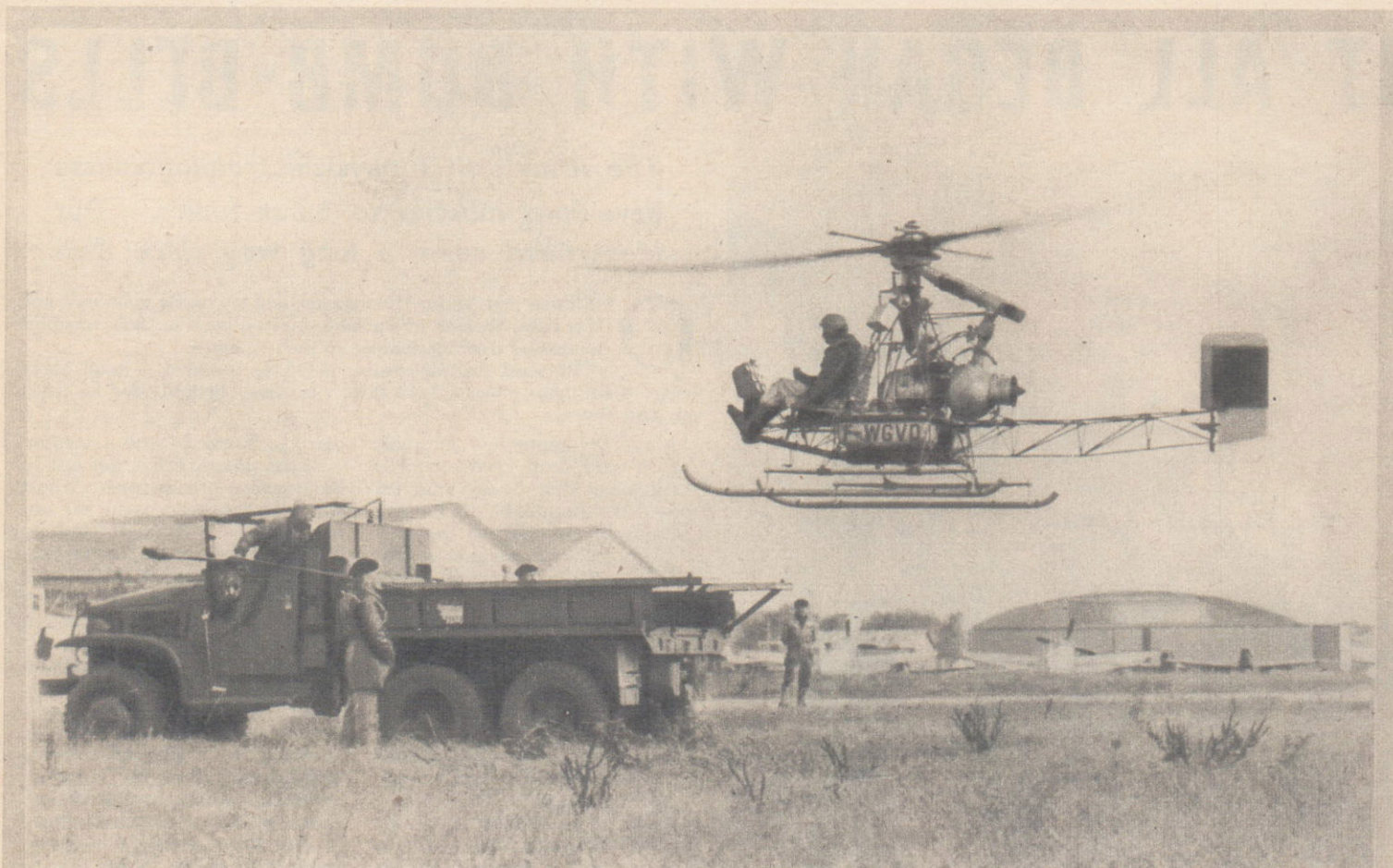
The latest thing in landing fields. This single-seater "Djinn" helicopter, fitted with skids, can land on and take off from a lorry, the smallest and most portable landing field yet invented. The demonstration was given recently in Paris.
