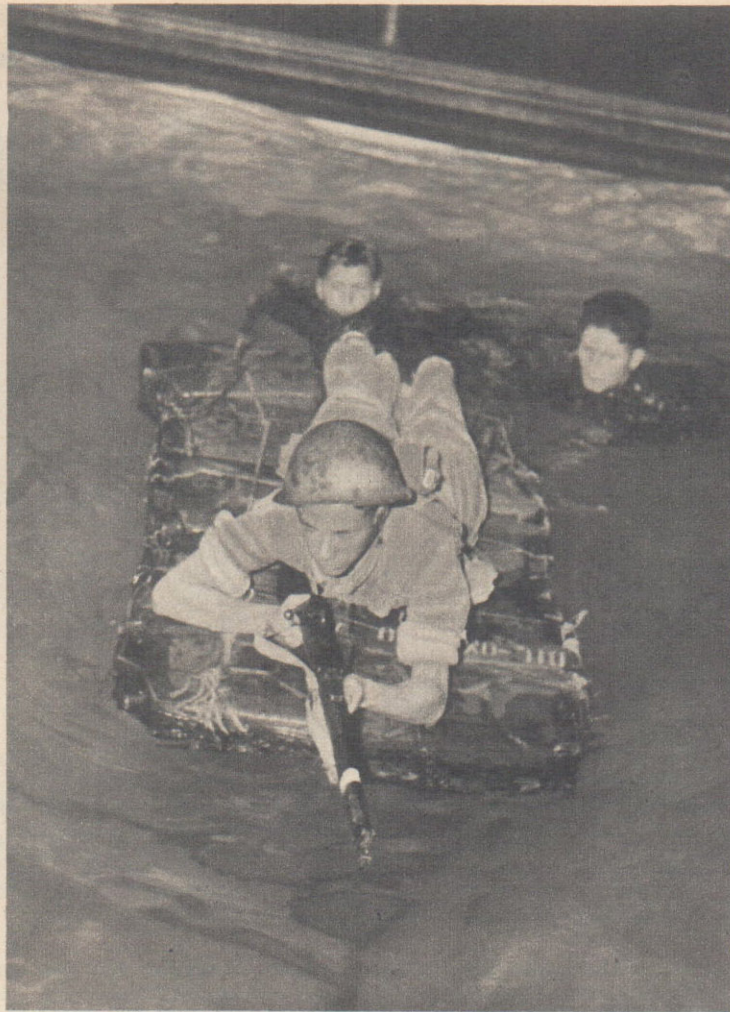
This two-manpower, jerrican-and-rope raft keeps a rifle firing.
