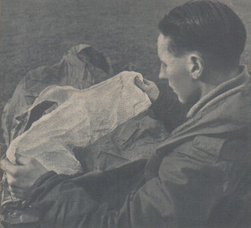
In order that radar operators may pick up the sleeve, metal mesh is incorporated in the fabric.
