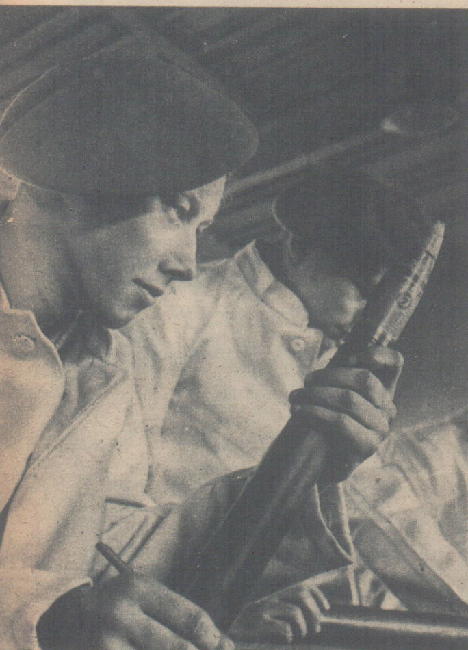
In the depot's laboratories a storeman records the details of a 40 mm round. Every new batch is checked for faults.
