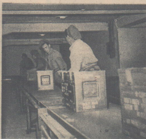
Ammunition moves along a conveyor belt which leads down a sloping shaft to join the main conveyor belt below. Below: a notice which speaks for itself.
