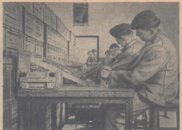
Left: Removing a suspect fuze from a mortar bomb — one of a batch giving prematures. The bomb is then passed through an aperture in the wall of boxes to the storemen (right) who plug the bombs. The wall acts as a rough shield against explosion.
