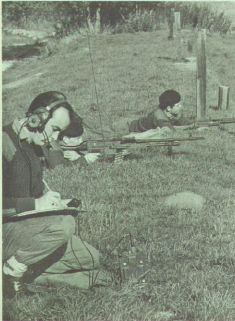
Clansman headset test—taking message during firing of machine-gun and rifles. Below: Mr Jack Dyer (fitter) and AQMS I Spencer examine SCAT.
