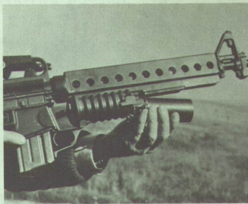
Above: Disposable type launcher (disposable barrel cartridge area target ammunition) attachment here seen mounted on the American M16 (Armalite) rifle.
