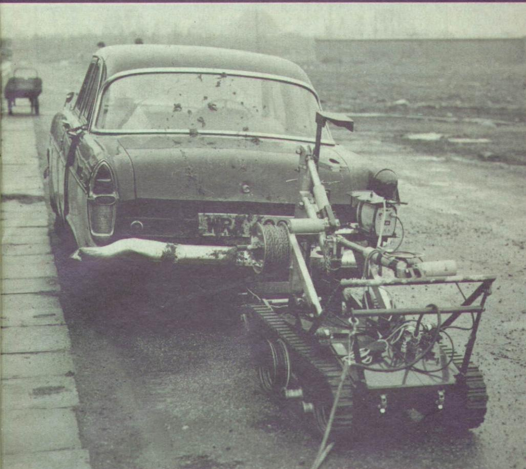
Above: Wheelbarrow robot attaches grab and tow rope to suspect car.
