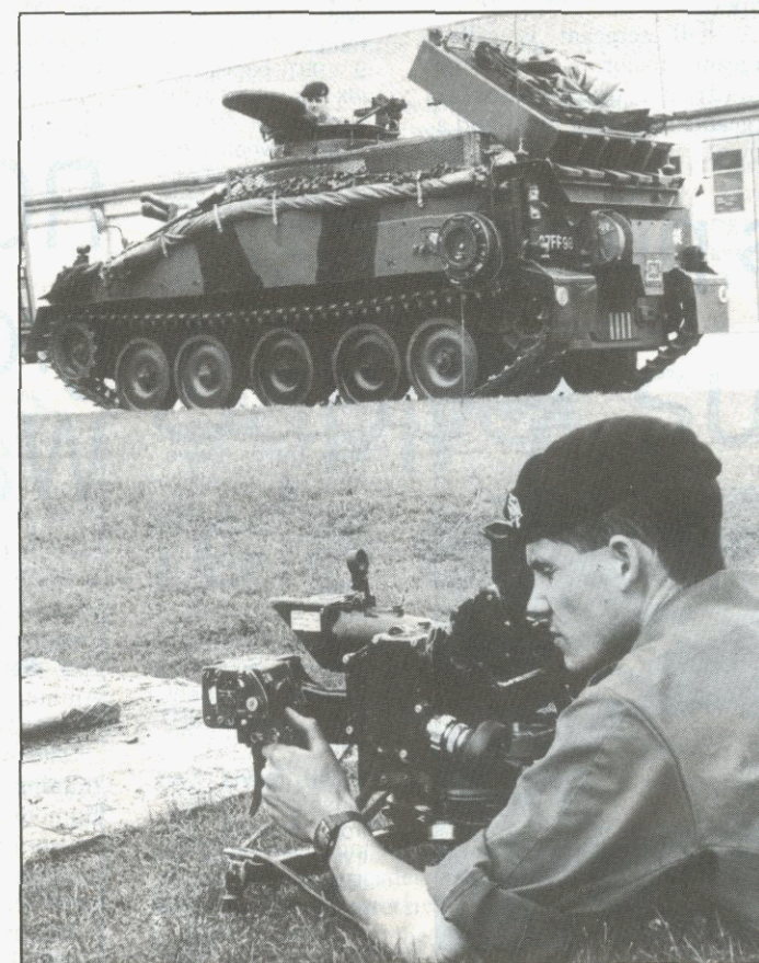
Tpr "Winker" Watson with the separated sight which enables Striker to fire by remote control
