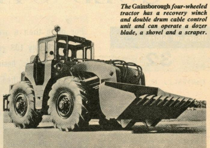
The Gainsborough four-wheeled tractor has a recovery winch and double drum cable control unit and can operate a dozer blade, a shovel and a scraper.
