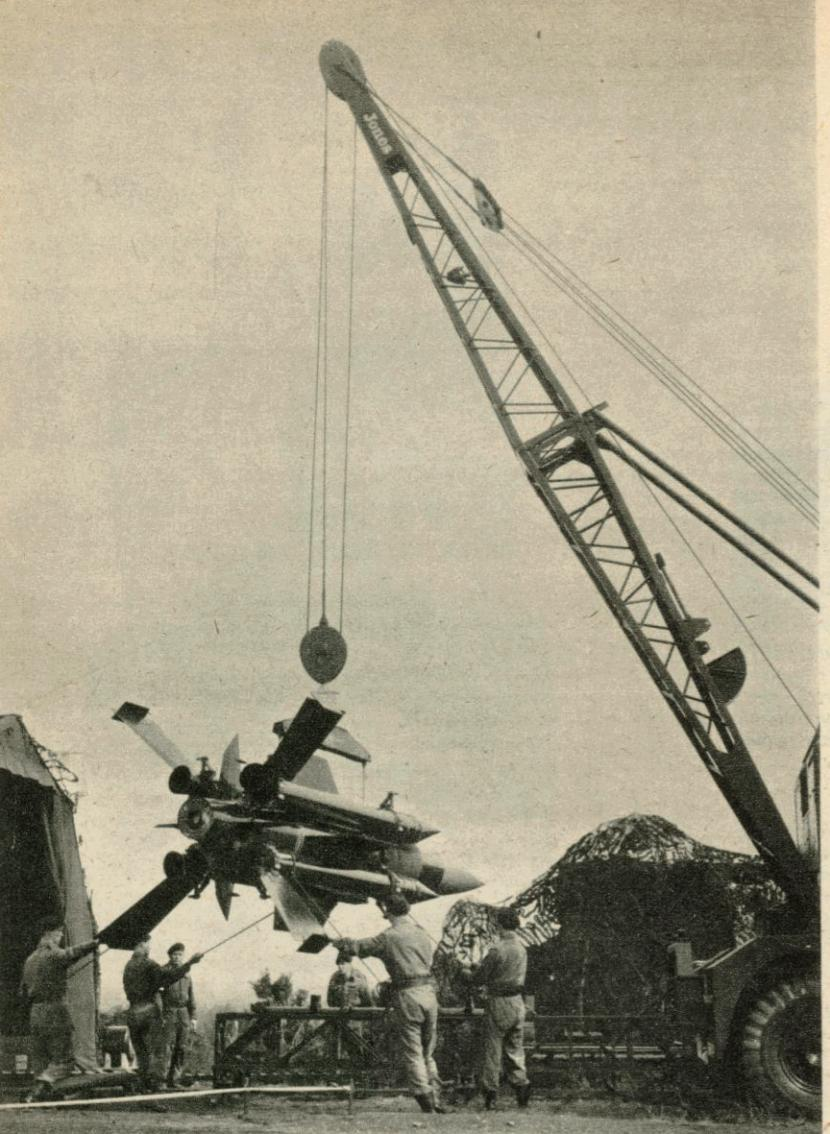
After the boosts and fins have been fitted and the missile tested in the forward assembly and test point, it is hoisted on to a transporter to be taken to the launching area. Below: Thunderbird is ready in position on the launcher.
