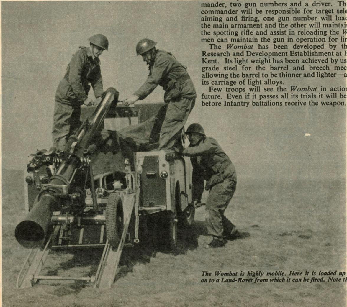
*The Wombat is highly mobile. Here it is loaded up a special ramp on to a Land-Rover from which it can be fired. Note the spotting rifle.*
