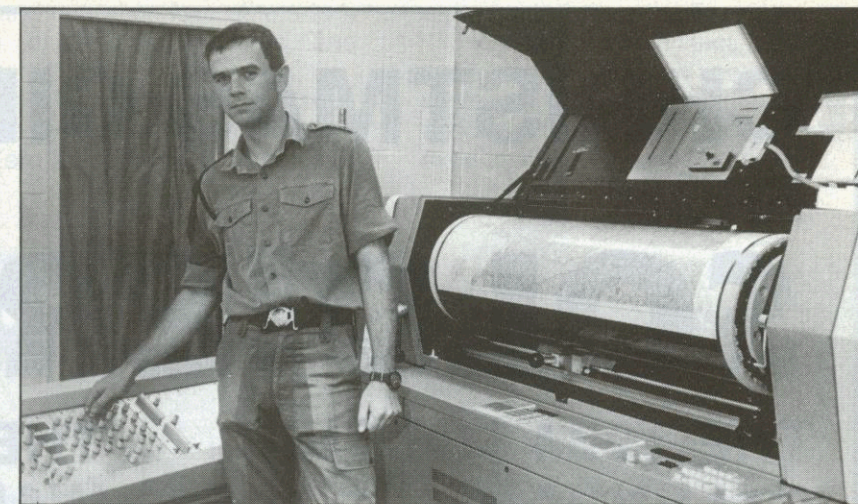
Above – LCpl Ray Powell operates a large scanner which splits a multi-coloured map into four colours. Maps used to be printed in a dozen or more colours, but four are quicker and simpler to reproduce
