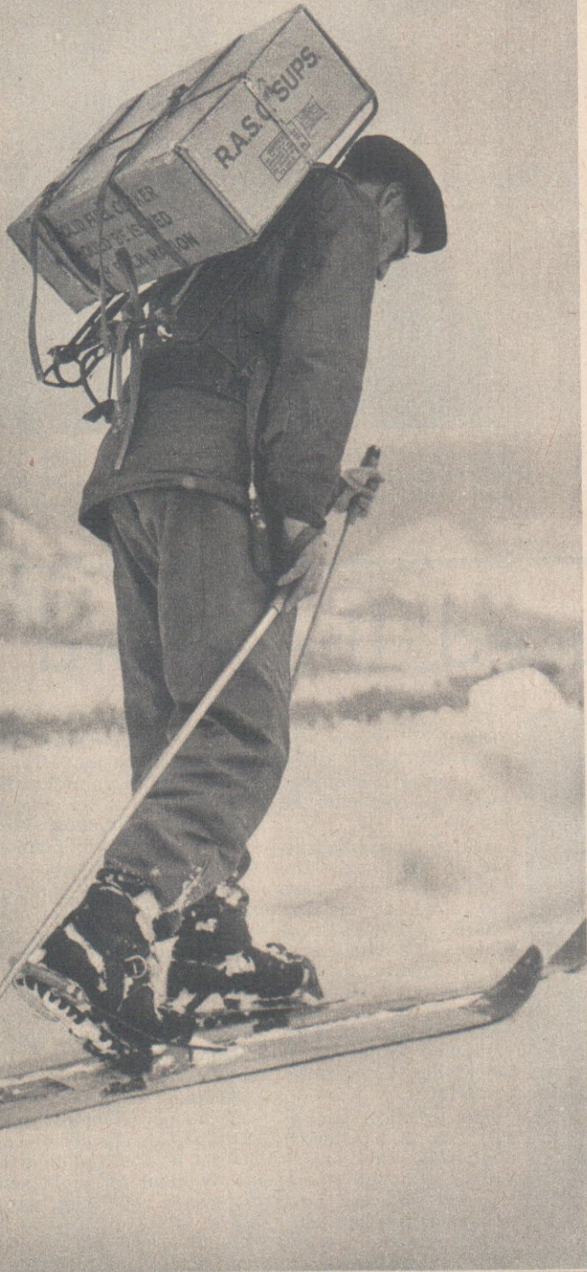
With a 65-pound box of rations strapped to a manpack carrier, Captain Alec Baines sets off on his skis. After 20 miles he will have a good idea whether the carrier is comfortable or not.
