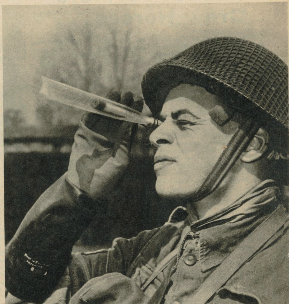
Left: Dressed for action, a member of a monitoring team with a survey meter. Note the rubber gloves, sweat rag (for keeping out radio-active dust) and the plastic waist bag for protecting metal articles like wrist-watches. Above: Reading the dosimeter.
