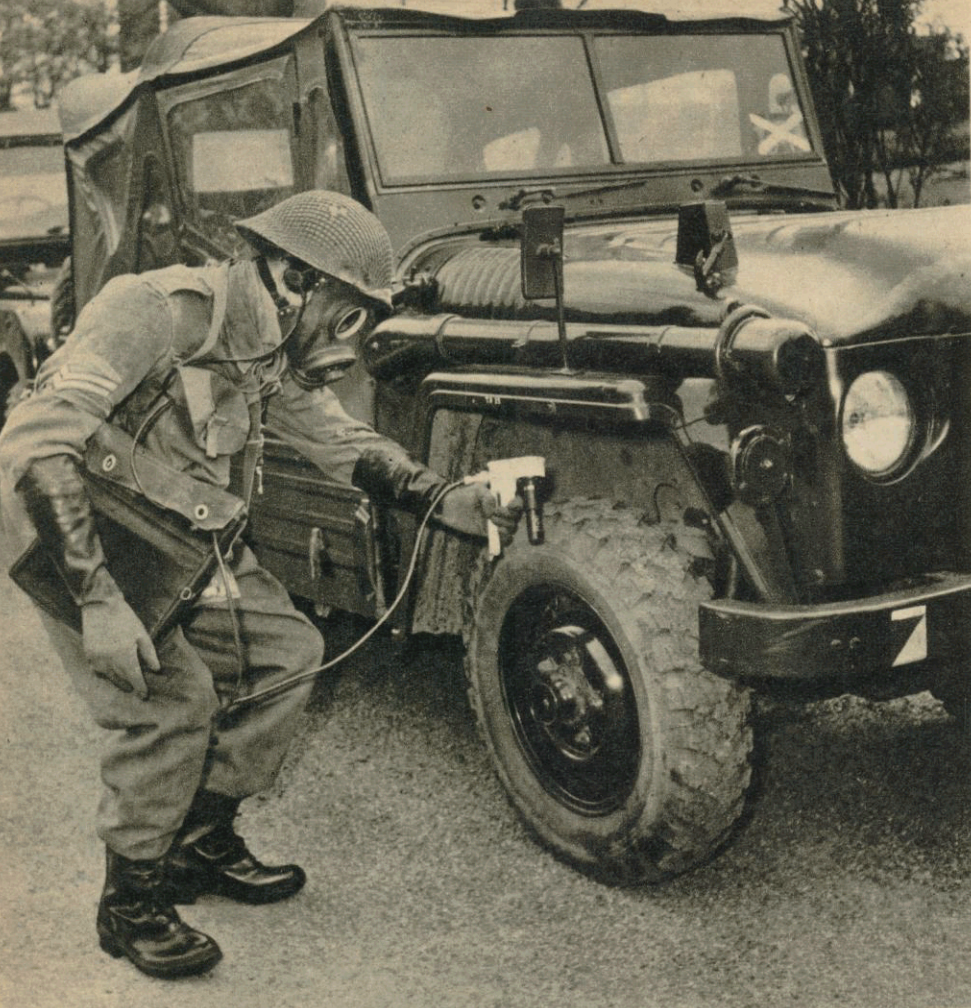
A Land Rover suspected of carrying radio-active dust is checked by a contamination meter. A Geiger counter measures the amount of infection.
