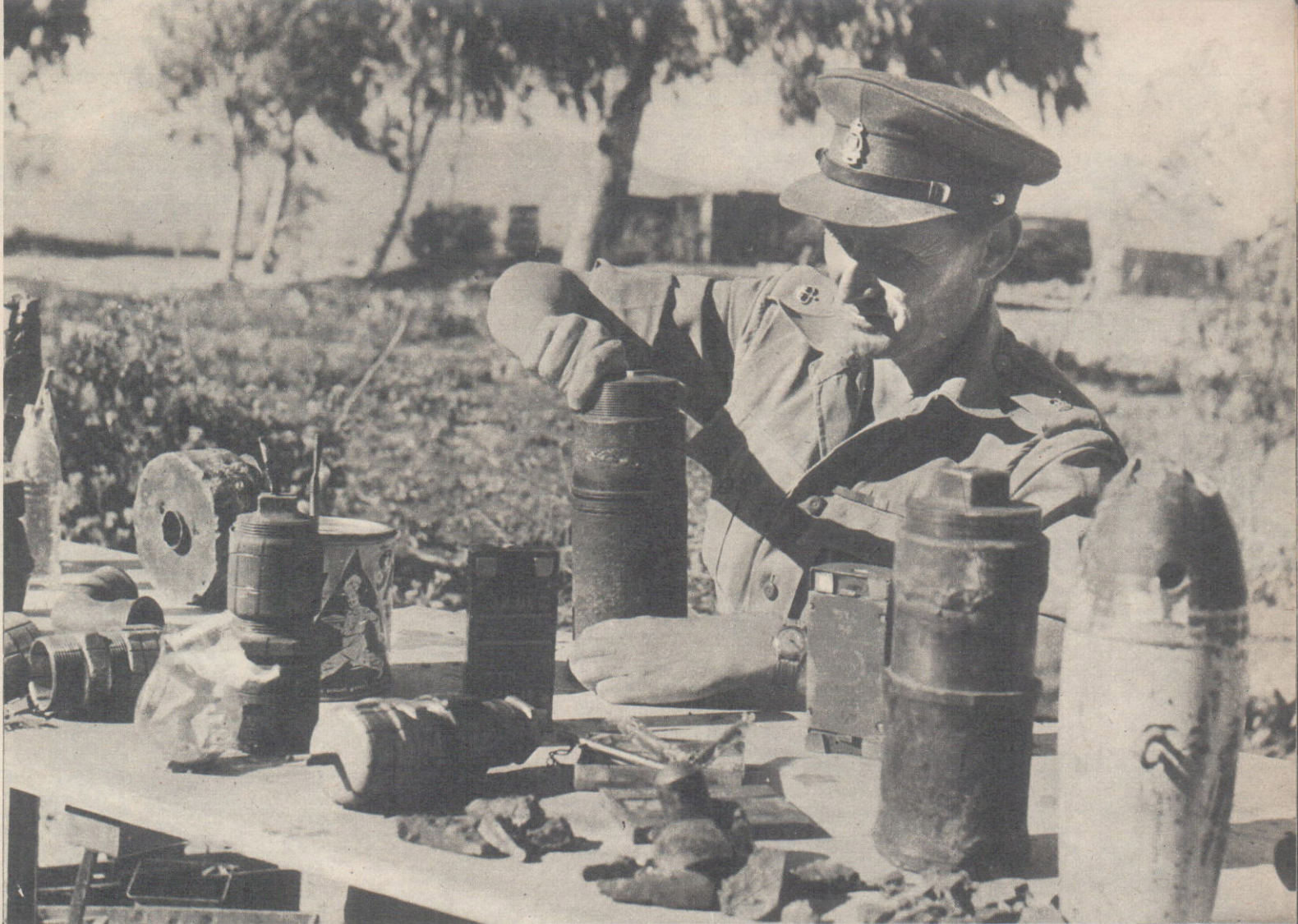
Major Harrison unscrews one of the home-made bombs designed to wreck buildings. They contain dynamite, with a time pencil inserted. Through lack of "know how" many are "duds." On the right is a Royal Air Force practice bomb, refilled with explosive with the object of using it to damage a bridge or a culvert. In the centre are two
