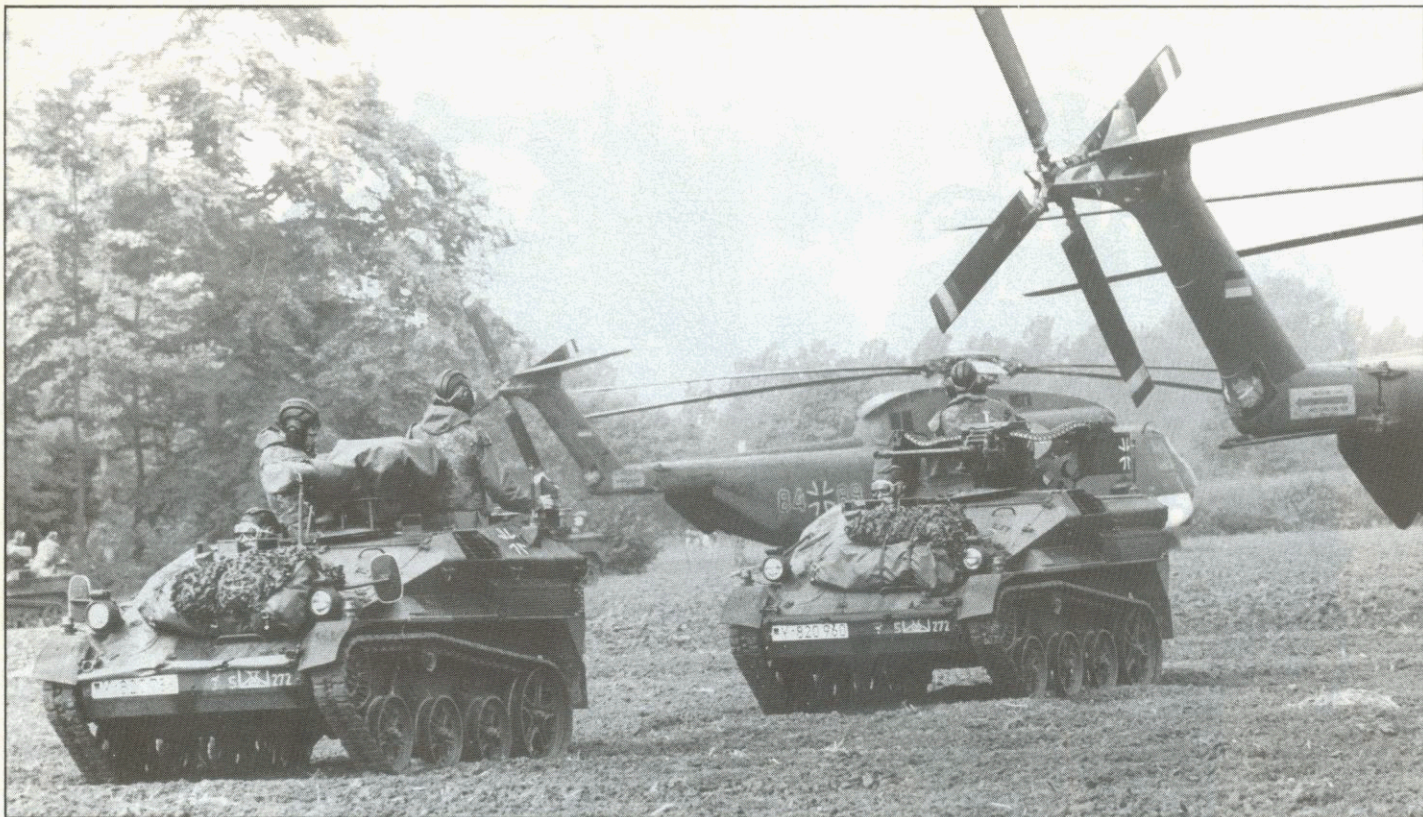
Two Wiesel air-portable armoured fighting vehicles reverse into the rear of a Luftwaffe CH53G helicopter. The Wiesel can be fitted with TOW missiles or a 25mm cannon
