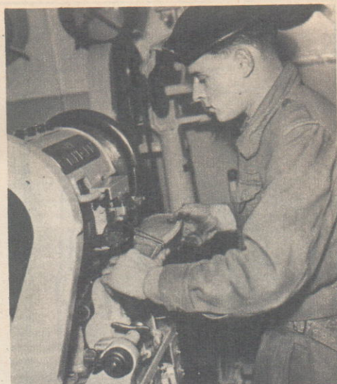
Below: Lance-Corporal A. J. Chappell and Private R. B. Crighton check the reproduction of a map printed on a Rotaprint machine.
