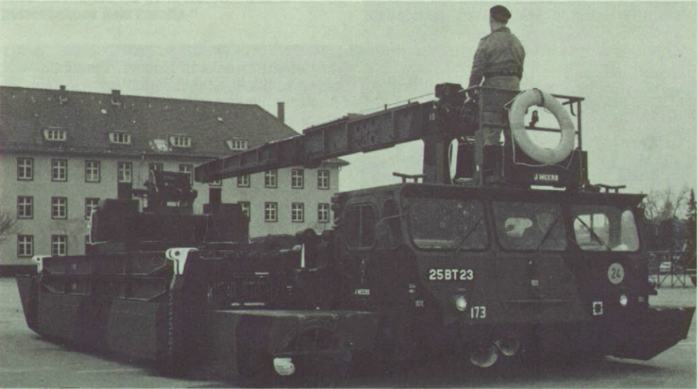
Ready for the road (above), the M2 amphibious bridging rig converts for marine use (below) by lowering side floats and retracting wheels.
