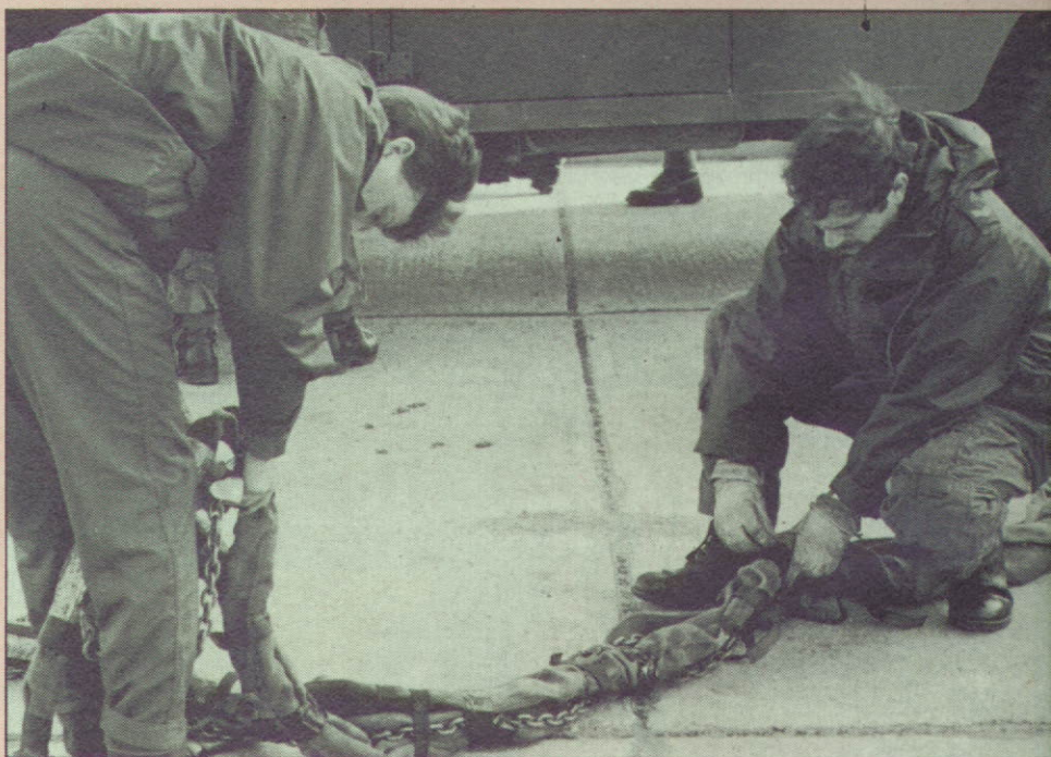
Hessian prevents chains damaging loads. ▶
