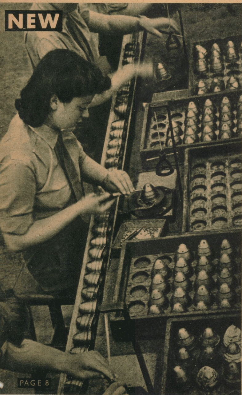
This was the method devised by the Motion Study experts. Fuzes came along on a roller feed. Each girl performed a clear-cut task. This way the job was done in 36 seconds.
