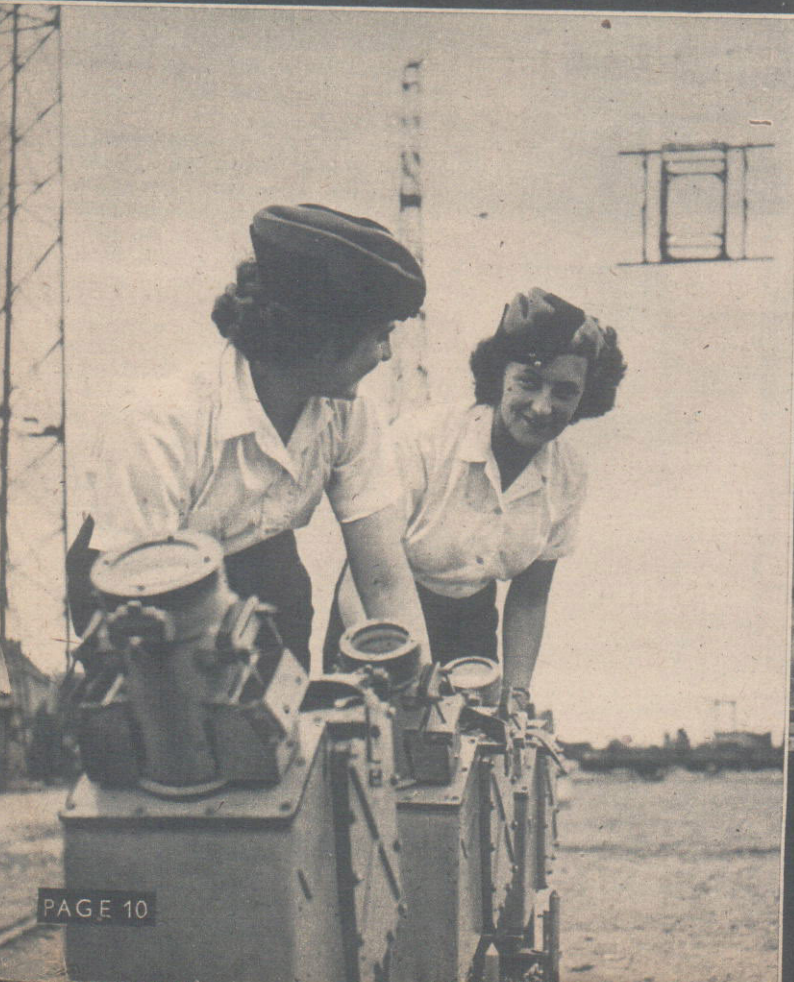
Corporal Shelagh Robinson wires up the frame of a screen through which a shell will pass; rupture of the frame is electrically recorded. Below: photo-electric cameras are lined up by Eileen McCulloch and Muriel Foulkes. Suspended in background is one of the target screens.
