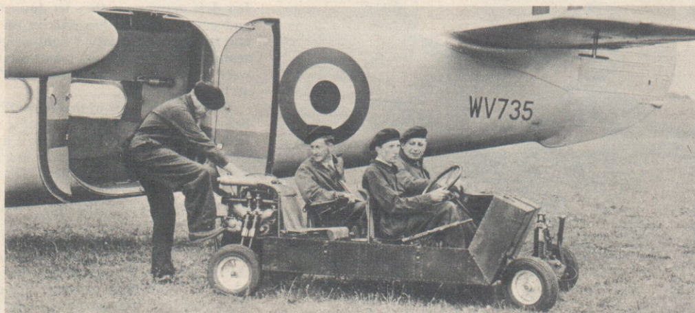
Only 45 seconds after touch-down, the Harrier is ready to move off. It has a top speed of 70 m.p.h. Note the driver's sub-machine-gun in its holder.
