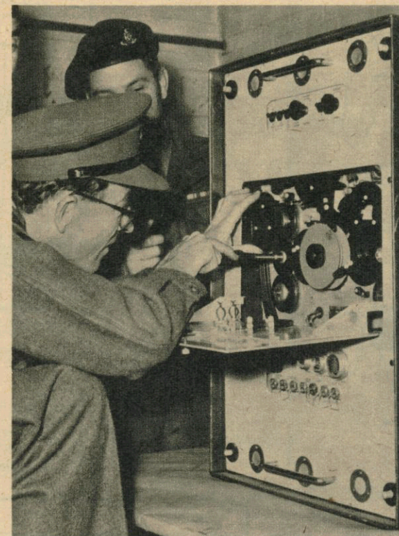
Major Hall adjusts the radar target simulator for which he invented a special cam to obtain an almost infinite variety of targets.
