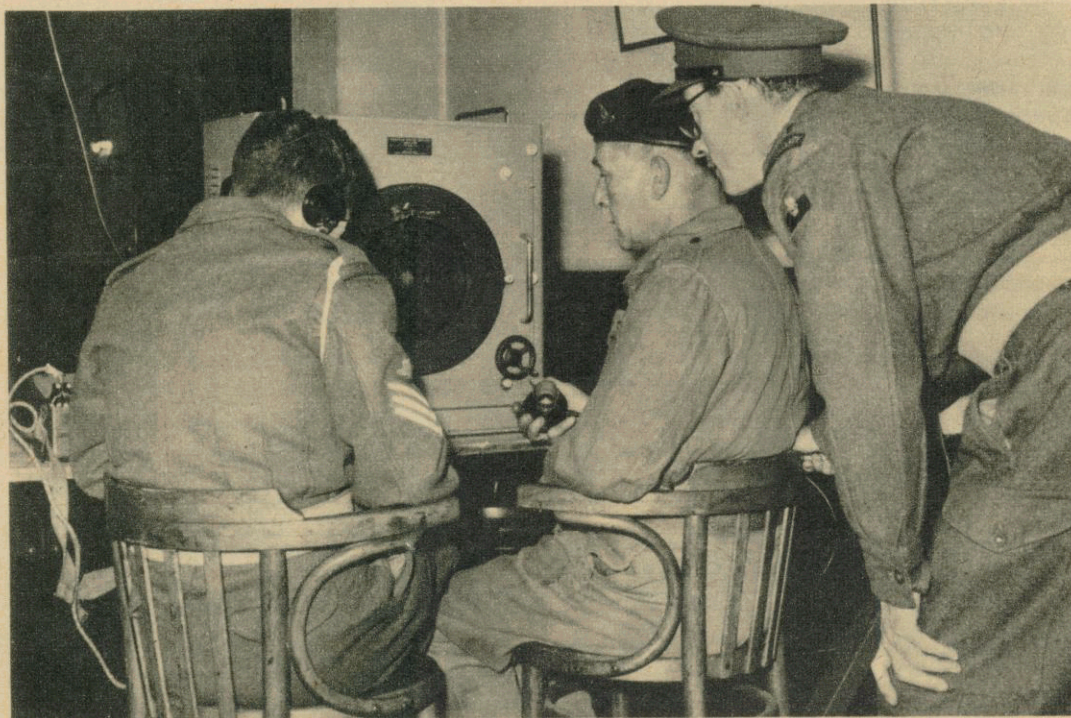
Above: The inventor explains his spotlight trainer to Battery Sergeant-Major A. Attwood and Sergeant K. Roberts, of 265 Light Anti-Aircraft Regiment, RA (TA). Below: The Hall Plan Position Indicator which simulates aircraft targets for radar operators. Several of these have appeared on television.
