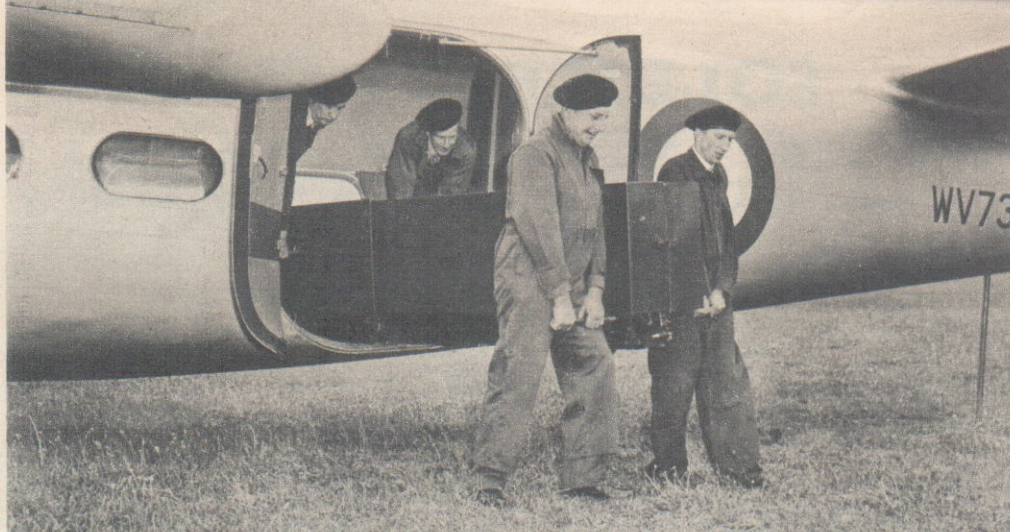
As soon as the plane halts the Harrier is manhandled to the ground by its own crew. No unloading tackle is needed as the coffin car weighs only 6\frac{1}{4} cwt.
