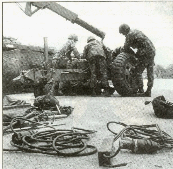
ONE – The lightweight launcher arrives on a lorry and has to be unloaded by crane and dismantled...
