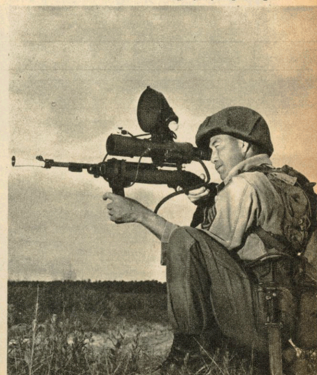
Below: STRAC is equipped with all the most up-to-date weapons, including this carbine rifle fitted with an infra-red sight for firing at night.
