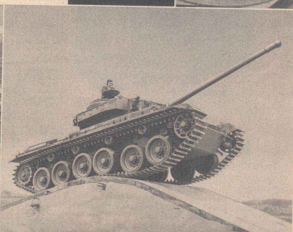
Below, left: The roof of a turret is welded on. Below, right: A finished tank is given a test over a concrete "hill."
