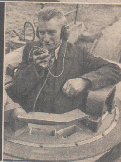
Wading test. The water is 4ft 9ins deep. The tank should stay in for half an hour without leaking.
