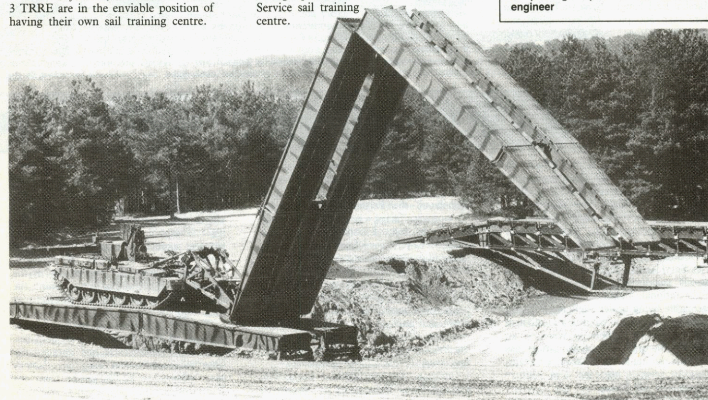
Bridge that gap. A Chieftain bridgelayer (AVLB) launching the 24 metre No 8 Bridge from a pre-launched No 8 Bridge supported on trestles
