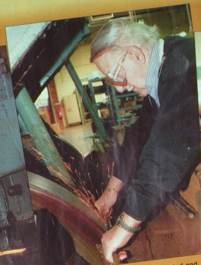
Hand-crafted: Billets of steel are heated and hammered to the correct thickness and length by Derek Brooks, left, while Carl Bandle, above, shapes, edges and points the blades
