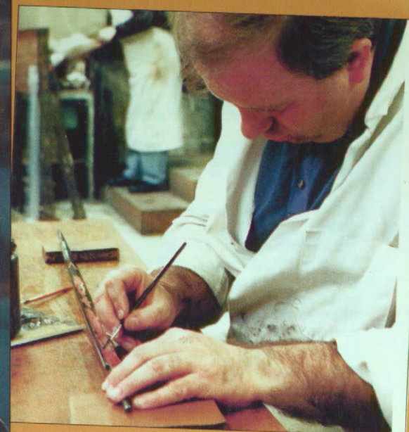
Craftsmen: Ray Humphries, above, undertakes the painstaking process of etching the blade, while Phil Black, above left, starts forming the hilt
