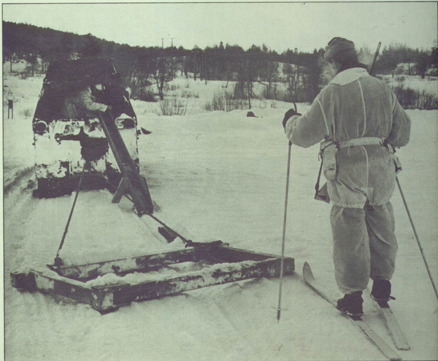
Above: Carrying one of the floats for Class 16 bridge and (right) assembling it in the bay. Below: Trialling minelaying by means of chute.
